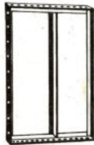
STANDARD PANEL 1000 mm-2500 mm (L) 100 mm-500 mm (W)
